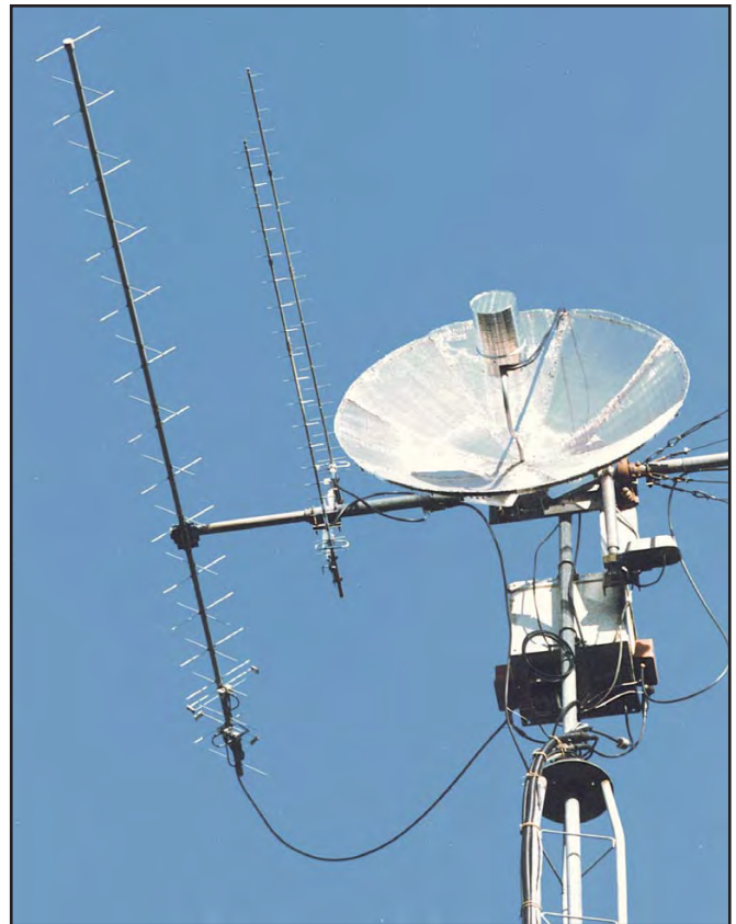
Fig 23.66—The completed and tower-mounted antenna system ready to go! The 40-W, 23-cm amplifier is enclosed in the box below the dish antenna.
