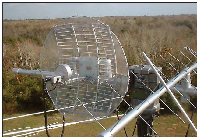
Fig 23.48 —K5GNA's "circularized" mesh modification of an MMDS dish antenna with helix CP feed and DEM preamp.
