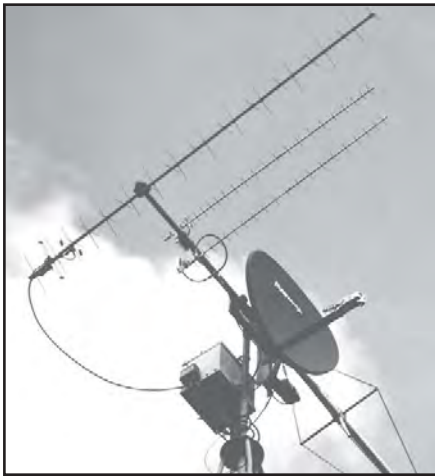
Fig 23.21 —Station antennas at WD4FAB. Mounted are T-B: M2 436-CP30, two stacked M 2 23CM22EZ, modified PrimeStar dish with homebrew seven-turn Helix feed antenna. The M 2 2M-CP22 antenna is off the bottom of the photo. See Fig 23.41 for details of the center section.
