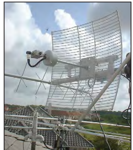
Fig 23.47 —K5OE's mesh modification of a MMDS dish antenna with helix CP feed and DEM preamp.
