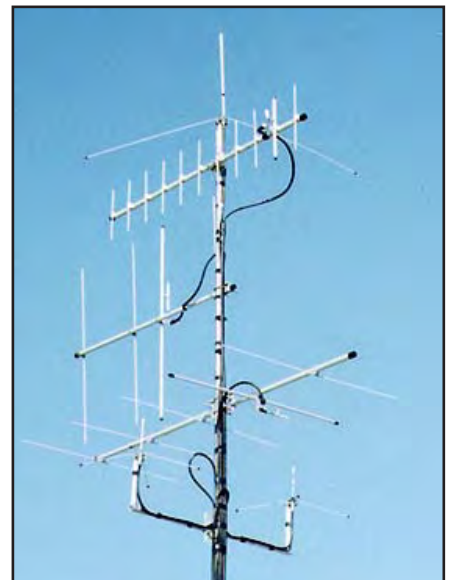
Fig 23.15 —Simple ground plane and Yagi antennas can be used for low-Earth-orbit (LEO) satellite contacts.
