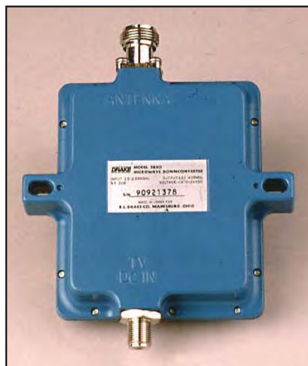
Fig 23.35 —S-band converter that was available from Drake, and easily modified for satellite service.
