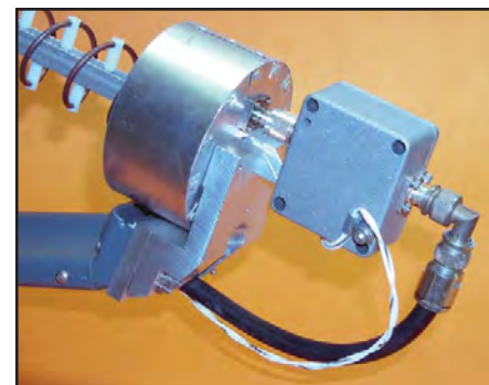
Fig 23.56—Mounting details of seven-turn helix and preamp.
