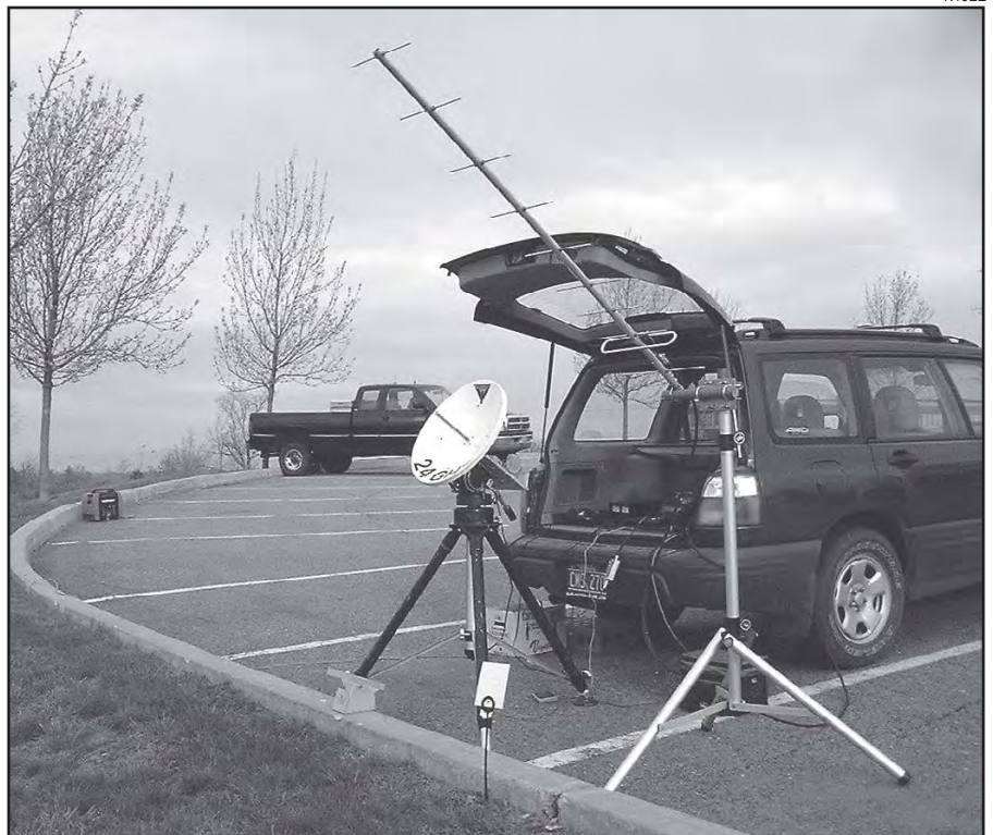
Fig 23.1—N1JEZ's portable microwave satellite station.
